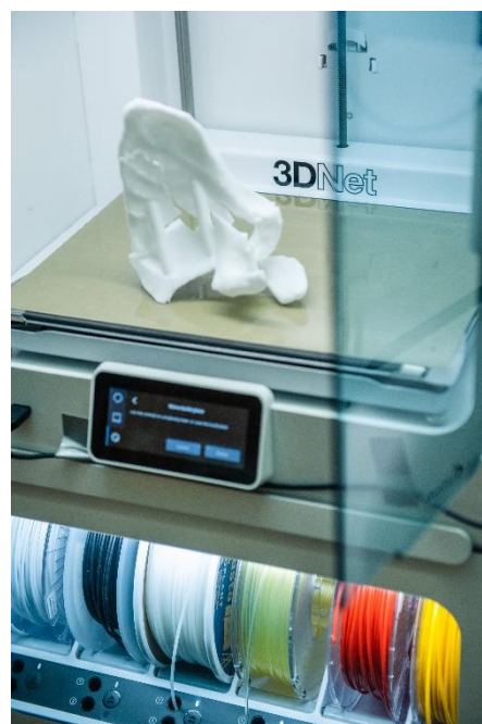
Figure 11: 3D printing of bone at the 3D lab in Glassgata in Ahus.
